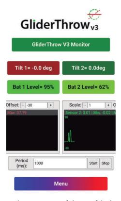
On this page you can see the percentage of charge of the batteries. Keep in mind that this value is an average estimate and should not be taken as an absolute value, however it will be useful to know the approximate state of charge of the battery.
