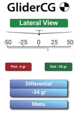
The numbered rule in the upper part will help us to identify in a simple way the weight deviation between both sides
