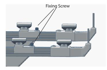
If, during the use of the GliderCG Scale, you wish to vary the distance of the supports to change between different models, once the distance has been modified you must perform a tare of the device as explained below.
