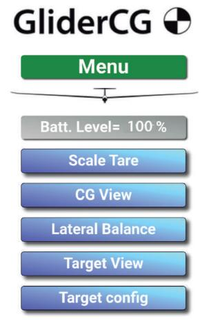
The first menu option "**Scale Tare**" allows you to zero the weight measurement or tare the scale.
