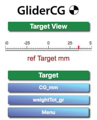
The numbered rule in the upper part will help us to visualize in a simple way the change in the position of the center of gravity between measurements.
