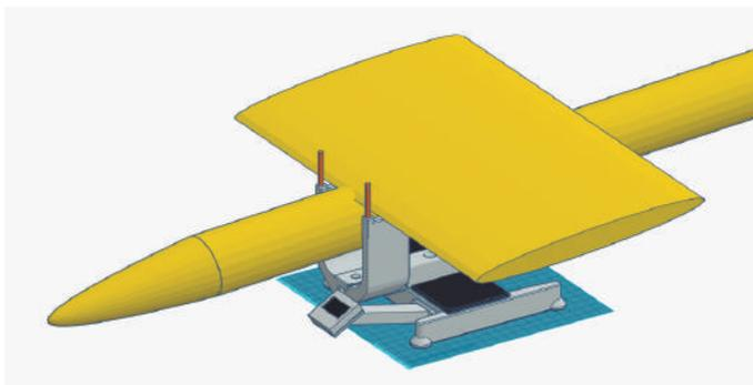
5° - Now the display shows an accurate reading of our CoG and the weight of our model.
