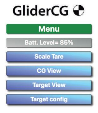
The first menu option "Scale Tare" allows you to zero the weight measurement or tare the scale.
